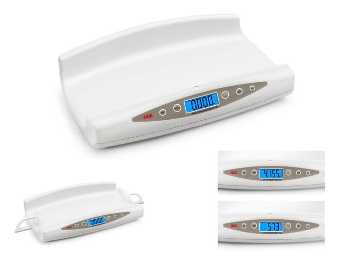
Electronic baby scale with large contoured baby tray. Exact reading down to 5 g with a total capacity of 20 kg. Optional available with integrated baby length measure – unique direct reading on the large backlit LCD display. Automatic zero setting, auto switch off, switchable auto-hold, back light display and optional length measure.
